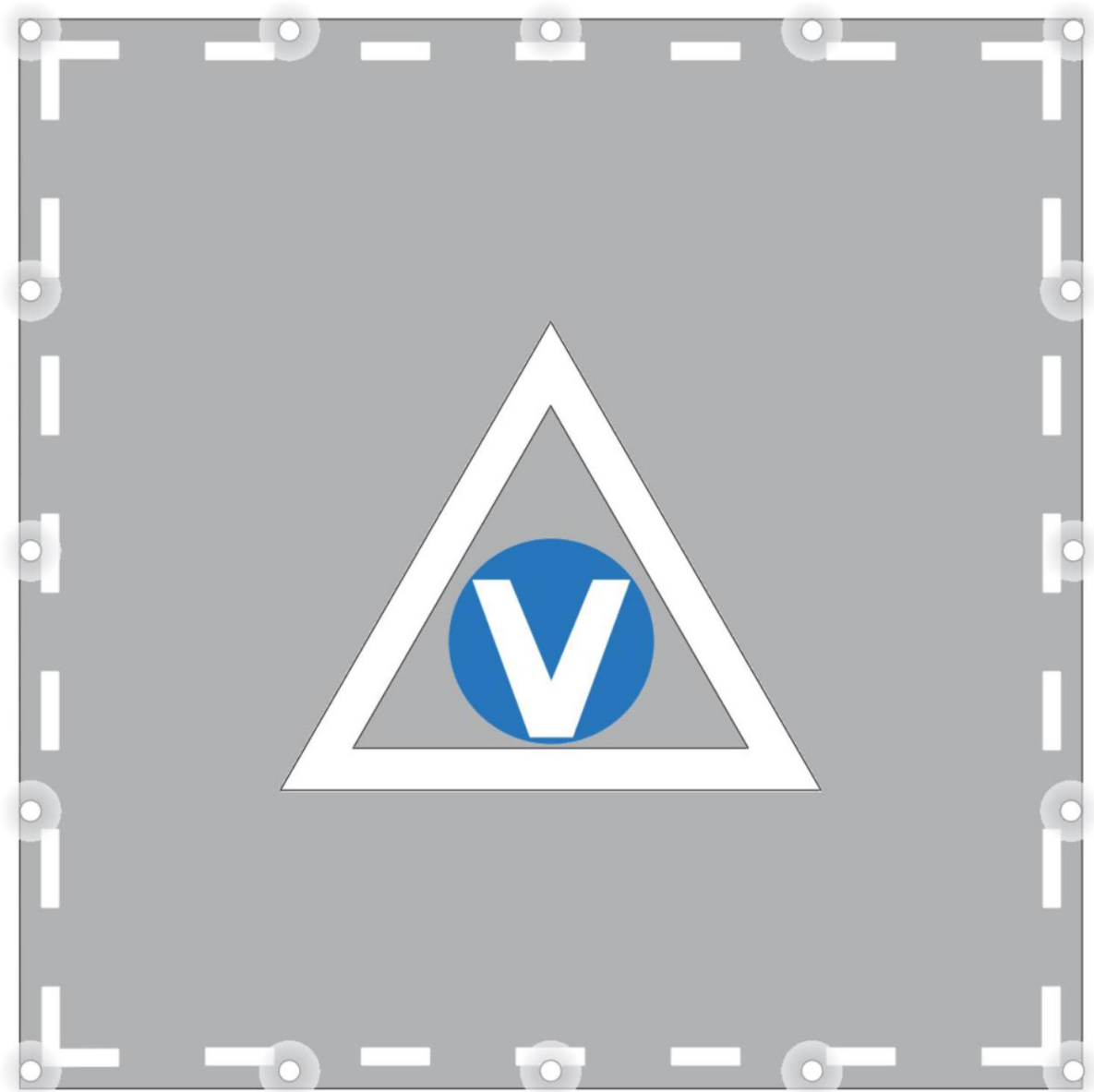
Figure 7-8. Lighting system for FATO at surface level
