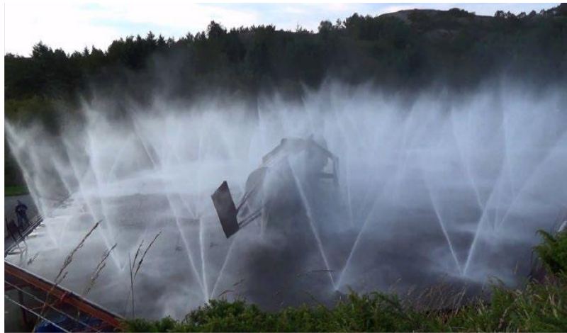
Figure 8-4 – Example of a dispersed pattern application on a solid plate heliport utilising DIFF
