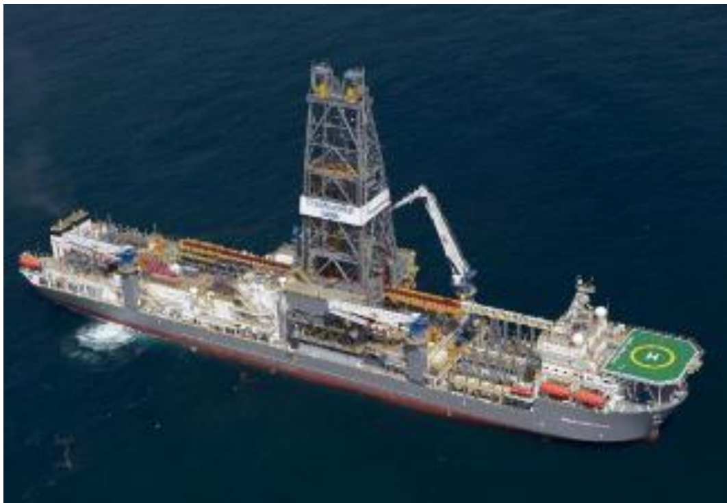
Figure A-5 High mounted bow helideck on a drill ship
