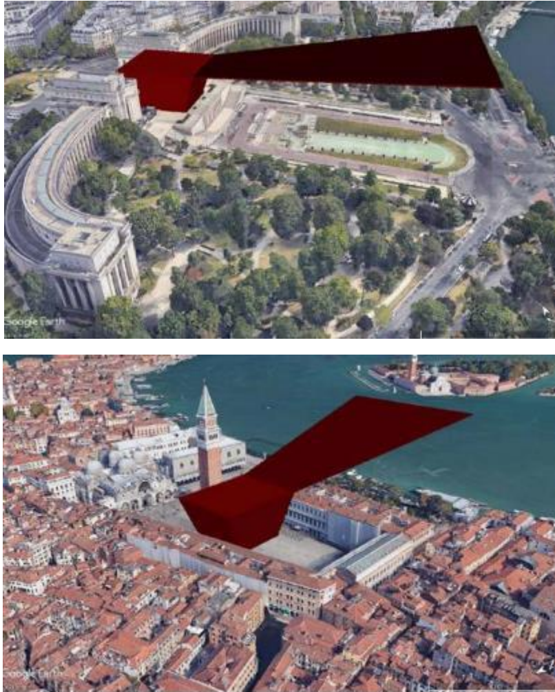
Figure 5-22. Examples of potential vertiports with Reference volume Type 1 (for illustration purposes only; the actual suitability has not been assessed)
