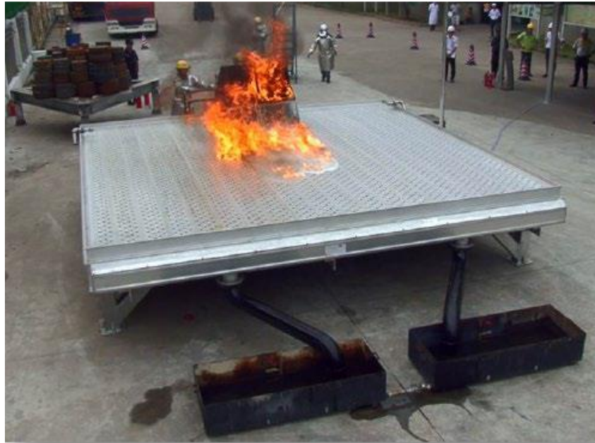
Figure 16-4: A fire test conducted on a passive fire-retarding surface using 200 L of burning fuel
