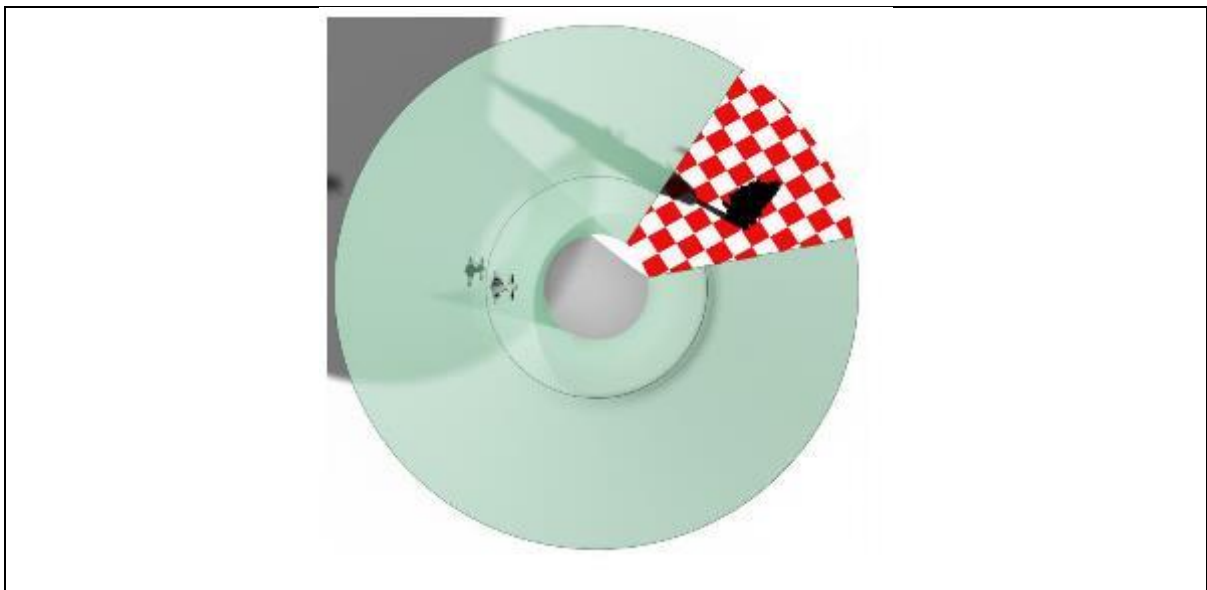
Figure 5-20. Vertiport obstacle-free volume with omnidirectional approach and take-off climb surface and prohibited sector — top view
