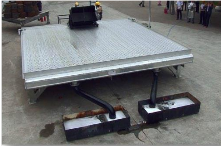
Figure 8-7 – A fire test on a passive fire-retarding surface (180 L of fuel is collected)
