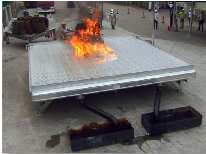
Figure 8-6 – A fire test on a passive fire-retarding surface (200 L of burning fuel)
