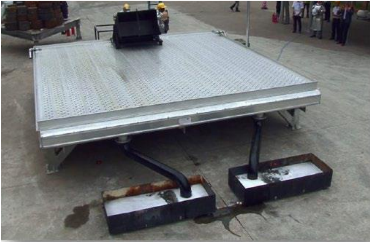
Figure 16-5: A fire test on a passive fire-retarding surface (180 L of fuel is collected)
